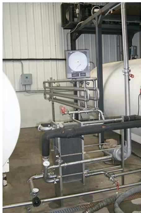
Since both types of pasteurizers have been shown to effectively destroy pathogens, either can be used. The critical point is to use the correct temperature and time for the type of pasteurizer chosen.
